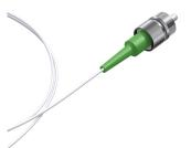
Single mode enhanced pigtails are used in telecom, datacom networks and also used for high speed metropolitan and access network. The single mode pigtail buffer conforms to IEC, EIA TIA or Telcordia standards. The single mode pigtails are terminated with optimized connectors each supplied with a protective cap on the zirconia ceramic ferrule.
